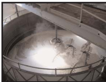
Cast iron mash tun dating back to 1881
